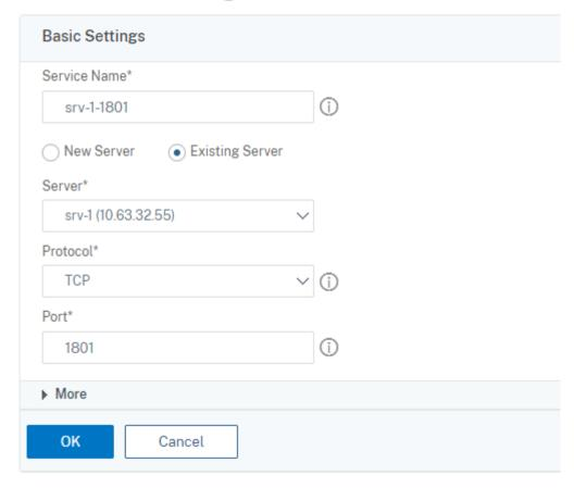
Bind the TCP monitor to the TCP load balancing service you just added.
