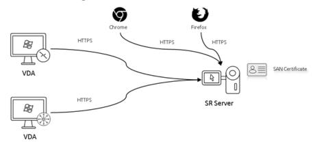
• When load balancing is in use, ensure that a SAN certificate is available both on Citrix ADC and on each Session Recording Server.
