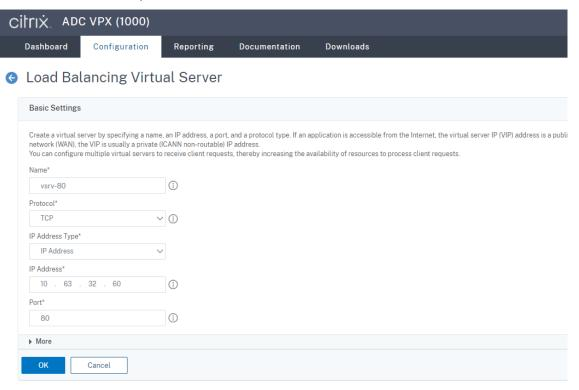
Bind each virtual server to the load balancing service of the same port. For example:
