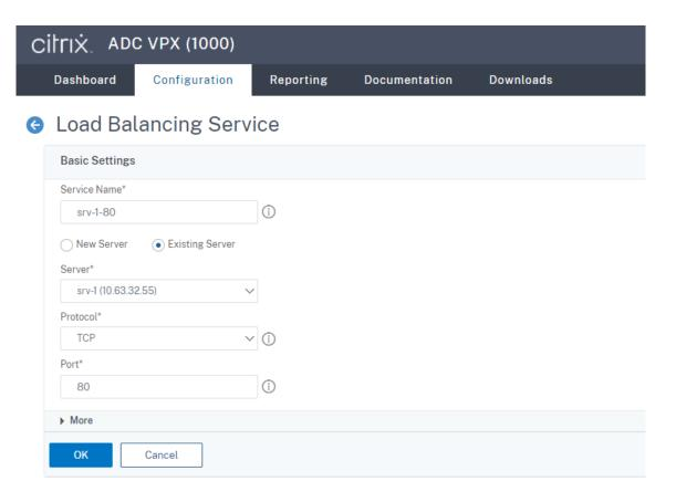
Bind the TCP protocol monitor to each load balancing service.
