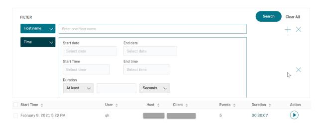
The **Time** filter consists of recording start date, start time, and duration.
