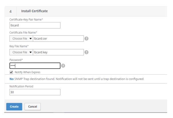
11. Bind a SAN certificate to each SSL load balancing virtual server.
