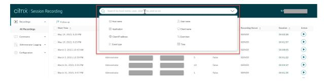
For example, after you select the host name filter, the following dialog box appears. Type in the host name (of the VDA where recorded sessions are hosted) and click **Search** to filter out irrelevant recordings and display only the relevant ones.
