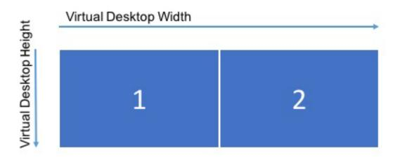
The diagram shows an out-of-the-box multi-monitor configuration with two monitors, each with a resolution of 2560×1600.
