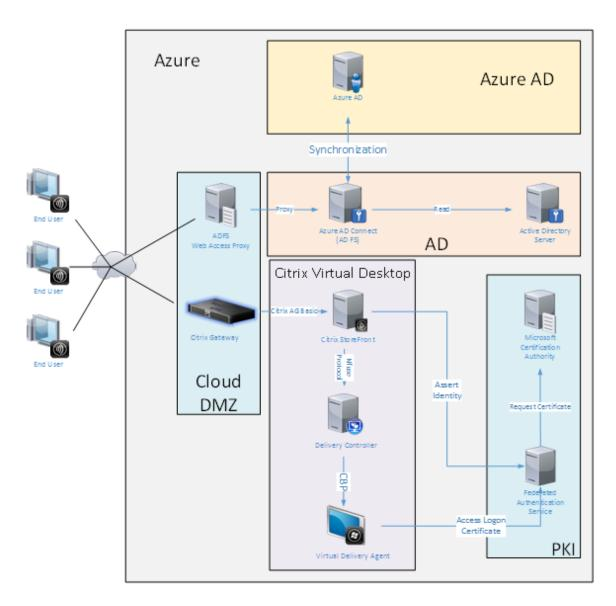
Secure connections and single sign-on, which would traditionally have been firewalled-LAN and Kerberos/NTLM authentication, are replaced in this architecture by TLS connections to Azure and SAML. New services are built as Azure applications joined to Azure AD. Existing applications that require Active Directory (such as a SQL Server database) can be run using a standard Active Directory Server VM in the IAAS portion of the Azure Cloud Service.
