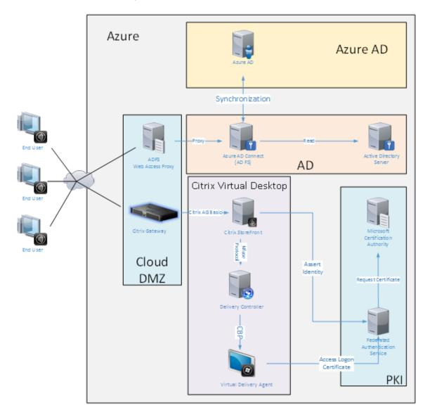
This deployment is an example where there is effectively no concept of "end users in the office."Laptops are enrolled and authenticate entirely over the Internet using modern Azure AD features.
