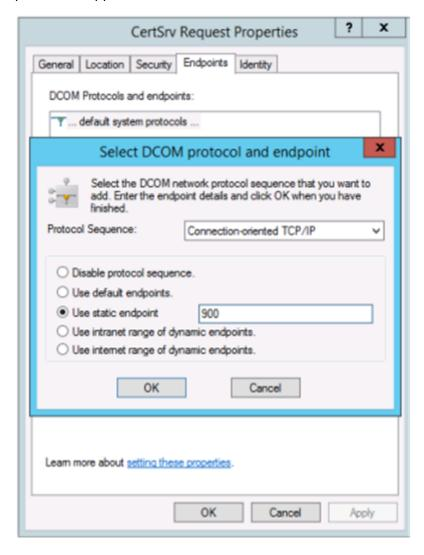
Change the "Endpoints" to select a static endpoint and specify a TCP port number (900 in the graphic above).
