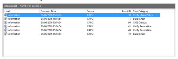
The final event log message shows Isass.exe on the domain controller constructing a chain based on the certificate provided by the VDA, and verifying it for validity (including revocation). The result is returned as "ERROR\_SUCCESS".
