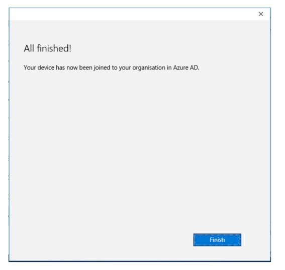
Verify that the Azure AD join was successful by restarting the machine and logging on, using the user's email address. When logged on, launch Microsoft Edge and connect to http://myapps.microsoft.com. The web site should use single sign-on automatically.
