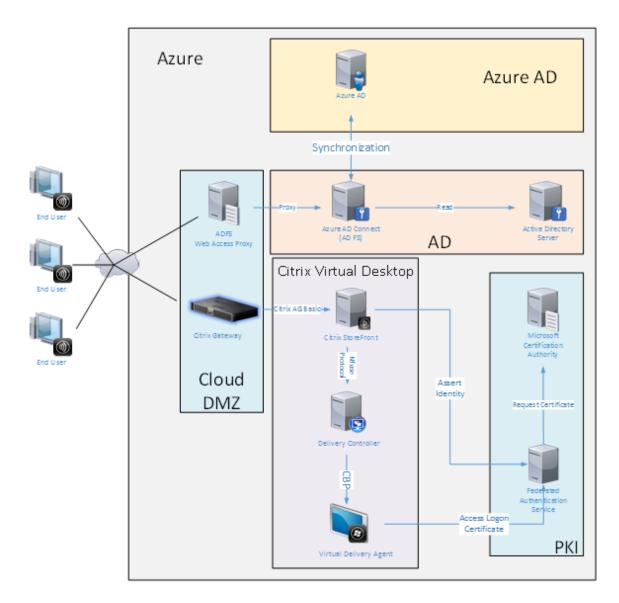
Secure connections and single sign-on, which would traditionally have been firewalled-LAN and Kerberos/NTLM authentication, are replaced in this architecture by TLS connections to Azure and SAML. New services are built as Azure applications joined to Azure AD. Existing applications that require Active Directory (such as a SQL Server database) can be run using a standard Active Directory Server VM in the IAAS portion of the Azure Cloud Service.
