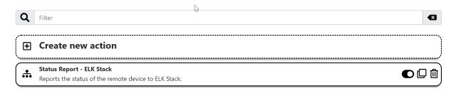
• Sending data to ELK Stack is configured by using a Web Request task.
