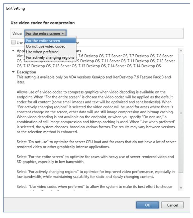
To confirm that H.264 compression is enabled for full-screen mode so that the SDA can function properly, see one of the following procedures.
