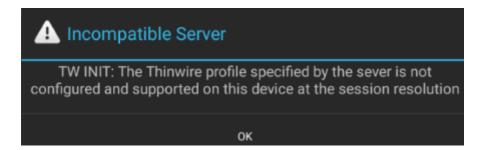
This error occurs if the graphic mode is configured as selective H.264 on the VDA. Screen casting performs better with the full-screen H.264 graphic mode. Reconfigure the graphic mode to **Full Screen** in **System Configuration** > **Connections** > **Workspace Hub**, or upgrade the VDA to version 1808 or later.
